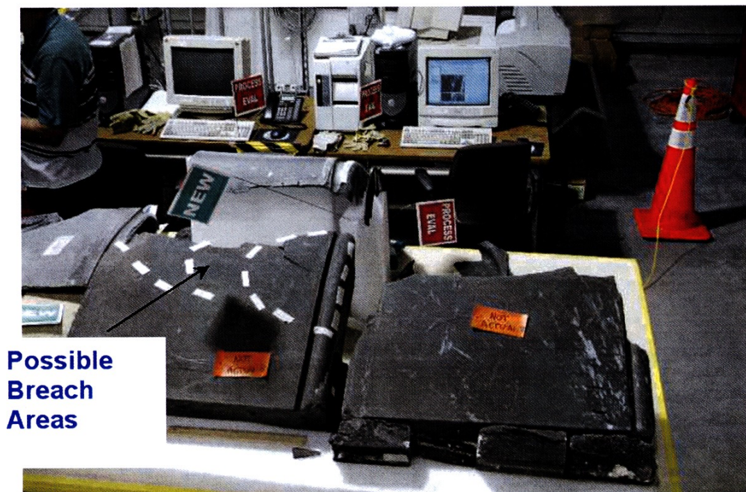
Figure 33: Probable Initial Breach in Panel 8.
